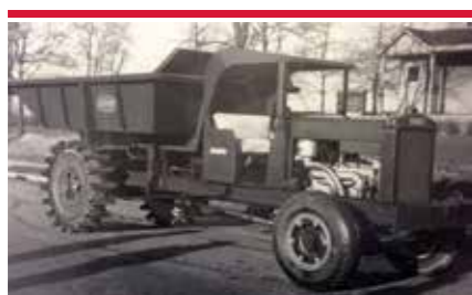
1934 The Model 1Z truck - considered to be the first true off-highway rear dump truck.
