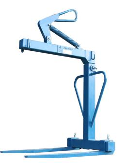
Fully self balancing even when unloaded, the CA103 has been designed to lift packs of bricks and pallets. The CA103 has adjustable forks and a frame to allow attachment of a safety net (NE100). The load height of these forks can be adjusted from 1100mm to 1600mm by a pin system.
