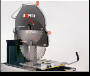
The cutting head is tilting and can be locked at the intended height.
