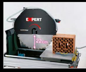
The cutting position with sliding carriage.
