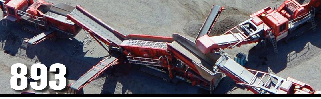
The New Terex Finlay 893 heavy duty screen is a robust high capacity machine, engineered and built for working in quarrying, mining, construction and demolition debris, topsoil, recycling, sand, gravel, coal and aggregate applications. The 893 features an aggressive forward-facing inclined modular configuration screen box with a 6.1 m x 1.8 m (20' x 6') top deck and a 5.5 m x 1.8 m (18' x 6') bottom deck and can accept bofar bars, speedharps, woven mesh, punch plate, tines and cascade fingers.
