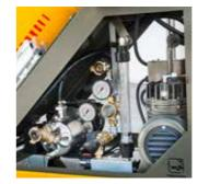
**Construction quality** Diaphragm compressor with an excellent output/ absorption ratio and low maintenance. Stainless steel self-priming water pump. All the components have been
