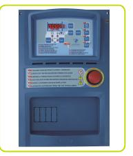
This version permits to control all the functions about a generator. It's built to monitor mono phase or three phase with neutral systems in alternate current; it permits to transfer the user's load on generator when the mains voltage is faulty. Conversely, as soon as AMF system detects the power grid, it stops the generator.
