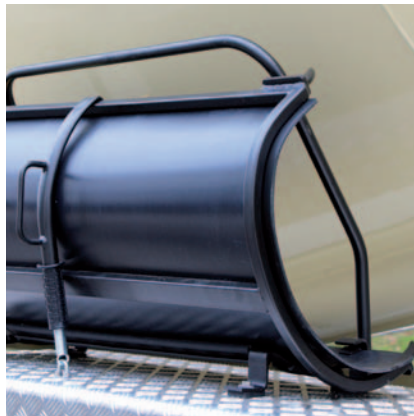
Plastic extension chute The low weight (per chute: approx. 9 kg only) helps in routine operations and saves weight in the overall superstructure. Up to two chutes can be hung one in another.
