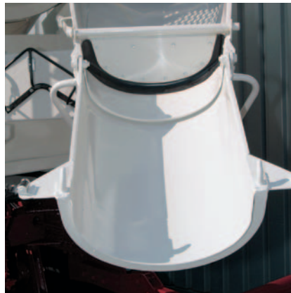
Retention flap for swivel chute It prevents residual concrete from escaping and thus soiling the road during driving.
