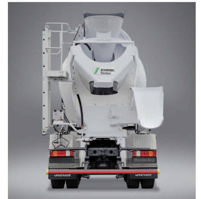
Ladder platform and ascent ladder made of aluminium (option) for further weight optimizing and comfortable handling.
