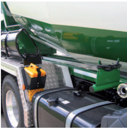
Attachment for flowing concrete pipes For transport of plastic pipes (DN 200) in lengths of 3 or 5 m provided by customer.
