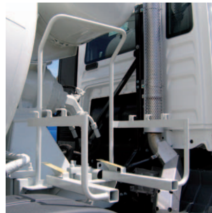
Support for mortar buckets Stacking device for mortar buckets with rapid-clamping closures.
