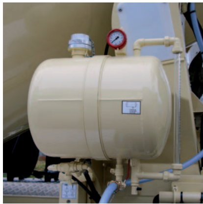
Admixture system in compressed-air version For filling plasticizer directly into the truck mixer. The pressurized admixture tank (tank size 60 l) is available in steel or stainless steel.
