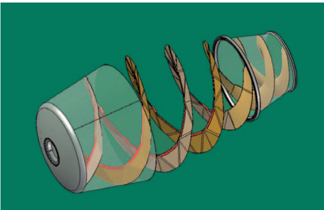
The new patented arrangement of mixing spirals makes for a considerably longer lifetime, even with highest load.
