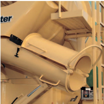
Hinged part made of steel Equipped with shackle for safe folding.
